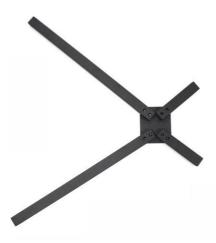
1.Put No.3 Long leg pole and No.4 short leg pole above No.2 fix panel as the above picture show
