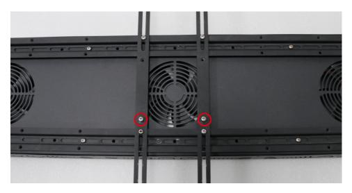
Fix No. 6 (fixing short rod) above No. 5 (fixing long rod) with No. 11 (M5 screw). Fix 2 # 11 (M5 screws) to the screw holes (arrow positions) in the same direction on # 6 (fixing short rod), and the screws only need to be locked in 2/3 of the way.
