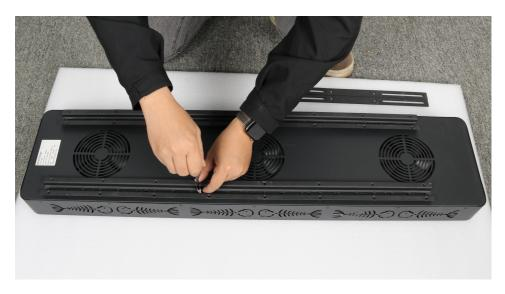
Match No. 5 (fixed long rod) with the fixing hole on the back of the therapy light, and fix it with No. 11 (M5 screw).
